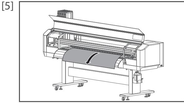
[5] From the front side of the printer, pull the media for approximately 1 m.
