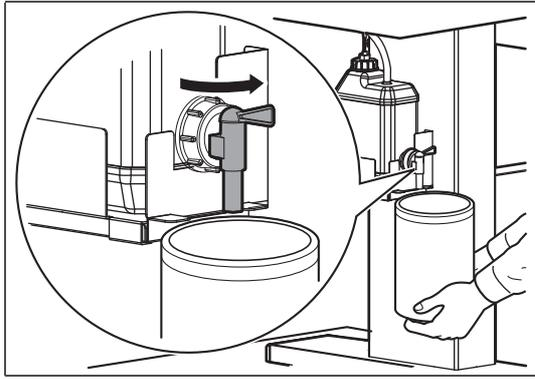
Open the waste ink valve and drain waste ink into the container.
