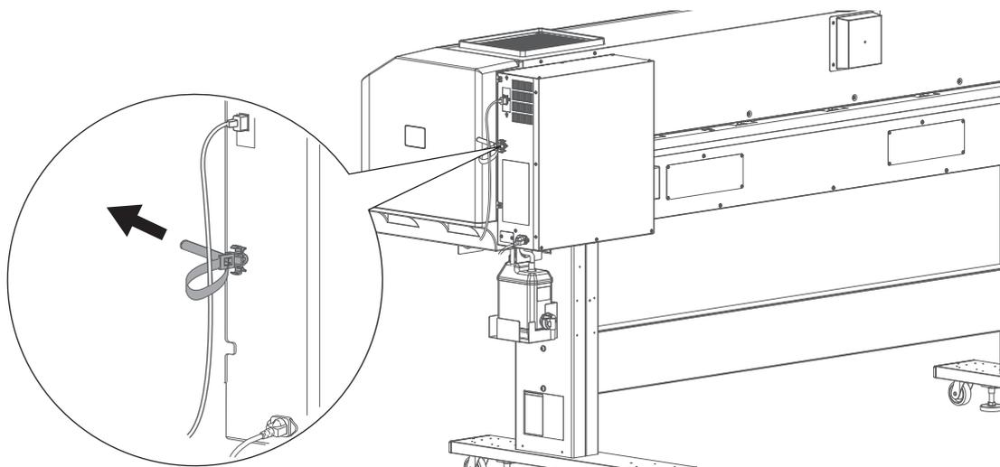
[4] Connect the Gigabit Ethernet cable to the computer.
