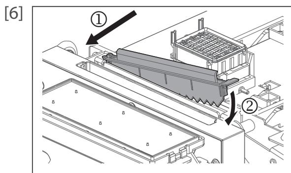
Attach an appropriate cleaning wiper to the wiper slot.
