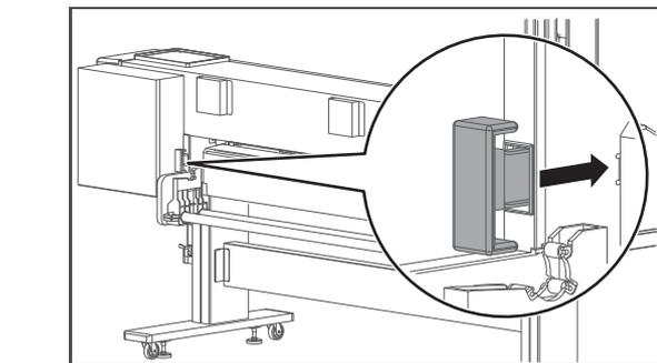
You can access to the media feed lever from the rear side of the printer.
