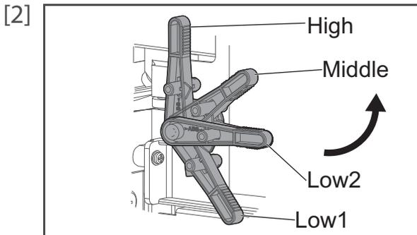
Use the head height adjustment lever (orange) to change the head height.
