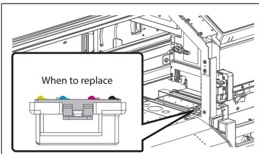
Check the absorption material for the flushing box.
