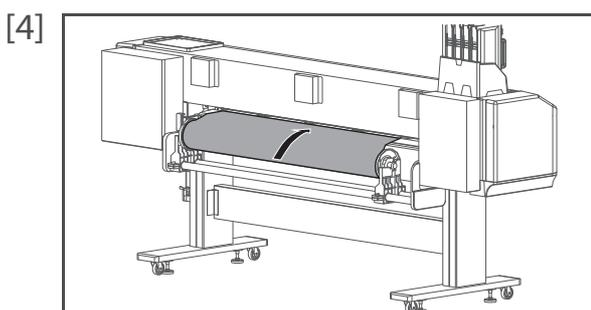
From the rear side of the printer, insert the front edge of the media into the media slot.
