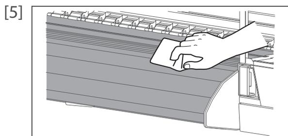
Use a soft cloth or paper towel slightly dampened with ethanol to clean off the ink on the platen, media guide and edge holders.
